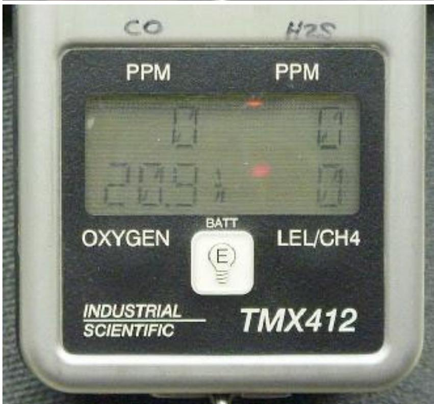
Example of a clean air display. Carbon monoxide (**CO**) and hydrogen sulfide (**H<sub>2</sub>S**) are in ppm; oxygen (**O<sub>2</sub>**) and lower explosive limit (**LEL**) readings are percentage values. The battery-life indicator is just right of the oxygen display (i.e., 20.9); each line represents about one hour of service remaining.
