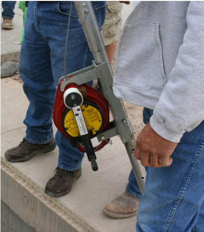
Checking the cable tension and inertial locking mechanism of the retrieval assembly.
