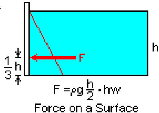
The simplest case is a rectangular gate of width  $w$ , and height  $h$ , whose top is a distance  $H$  below the surface of the water.
