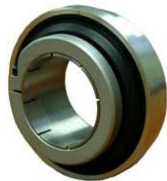
Mechanical seals are ideal for pumps that operate in closed systems (such as fuel service and air-conditioning, chilled-water, and various cooling systems). They not only conserve the fluid being pumped, but also improve system operation. The type of material used for the seal faces will depend upon the service of the pump. Most water service pumps use a carbon material for one of the seal faces and ceramic (tungsten carbide) for the other. When the seals wear out, they are simply replaced.
