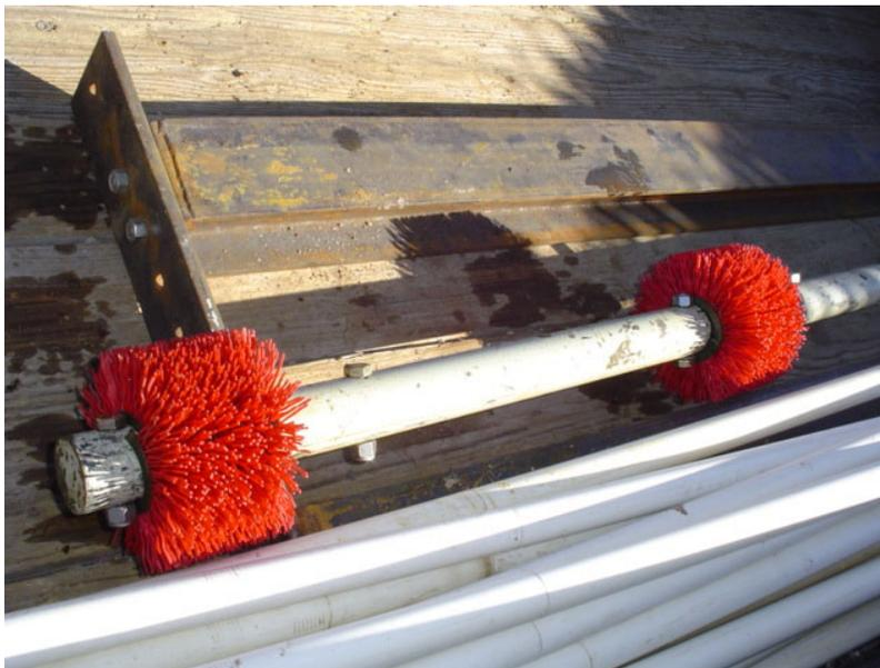
This brush is used to dislodge debris inside well casing. Just a big toilet cleaning brush.
