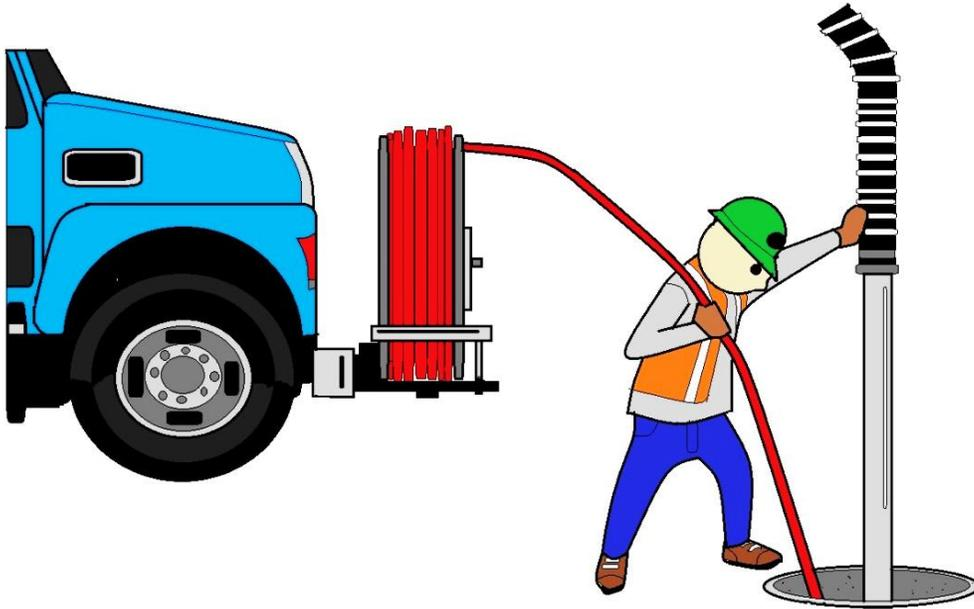
**USING A VACUUM TRUCK TO CLEAN SEWER**
