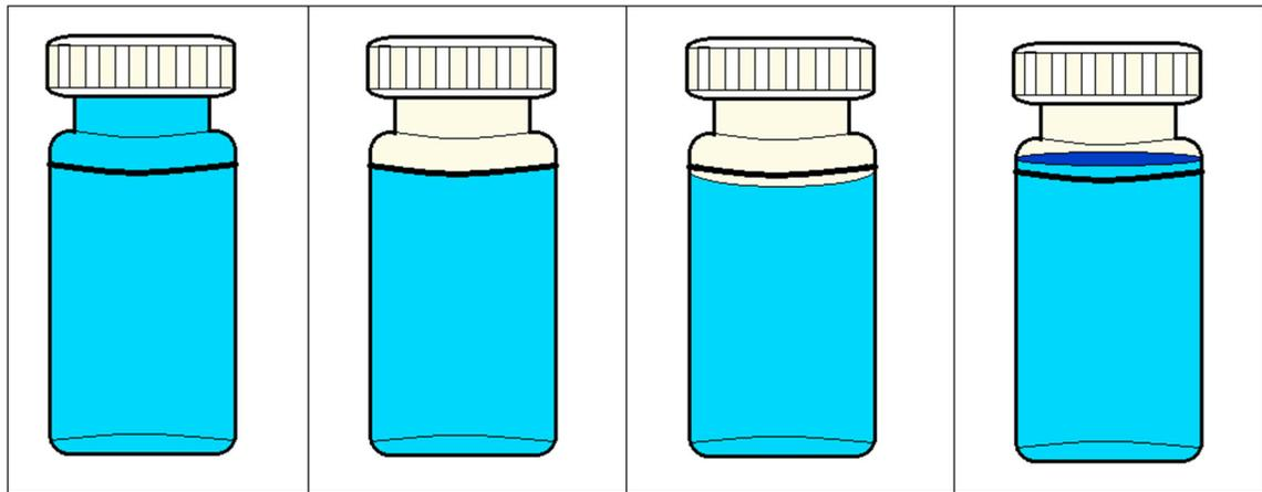
OVER FILLED      CORRECT (100mL)      INCORRECT (97mL)      CORRECT
