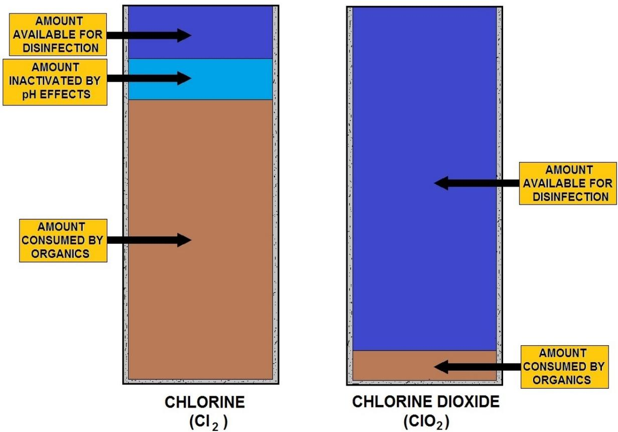
THE DIFFERENCE IN USING CHLORINE AND CHLORINE DIOXIDE AS A DISINFECTANT
