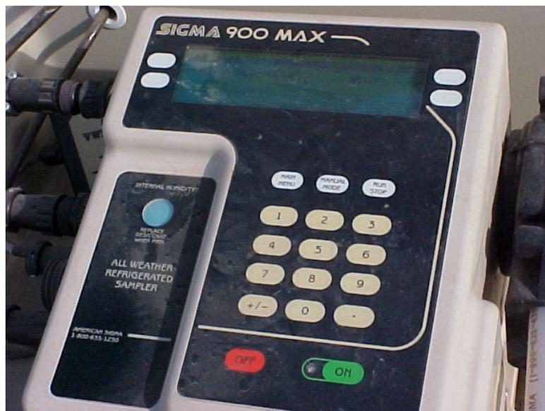
The Refrigerated Automatic Sampler will have a Data programmer that will allow you to set the time to collect the sample or samples. This machine can also measure the amount of the sample. These can also be used for the collection of composite samples. Sometimes you will see a pH probe with real-time readings sent to the Operator's Command Center. This is a common sight for most wastewater plants and SIUs.
