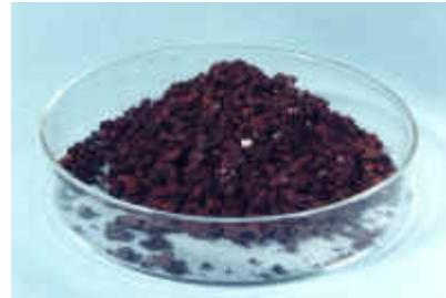
The water treatment residues, with and without cement encapsulation, passed the standard US EPA TCLP leach test for landfill disposal.
