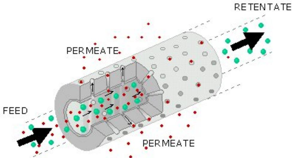
Transport through the membrane is performed by a pressure difference, a concentration difference, a chemical or electrical potential difference as a driving force. The membrane itself forms a semi-permeable barrier through which some particles are transported faster than others, so that a separation occurs.
