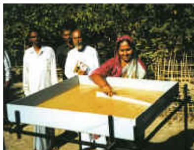
After solar oxidation the arsenic contaminated water is transferred into the CRC-ANSTO designed settling urn. After settling overnight, the urn provides the convenience of 'clean drinking water on tap' to a Krishnapur villager.
