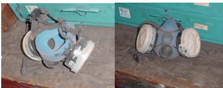
Unacceptable maintenance and storage (OSHA Violation)
