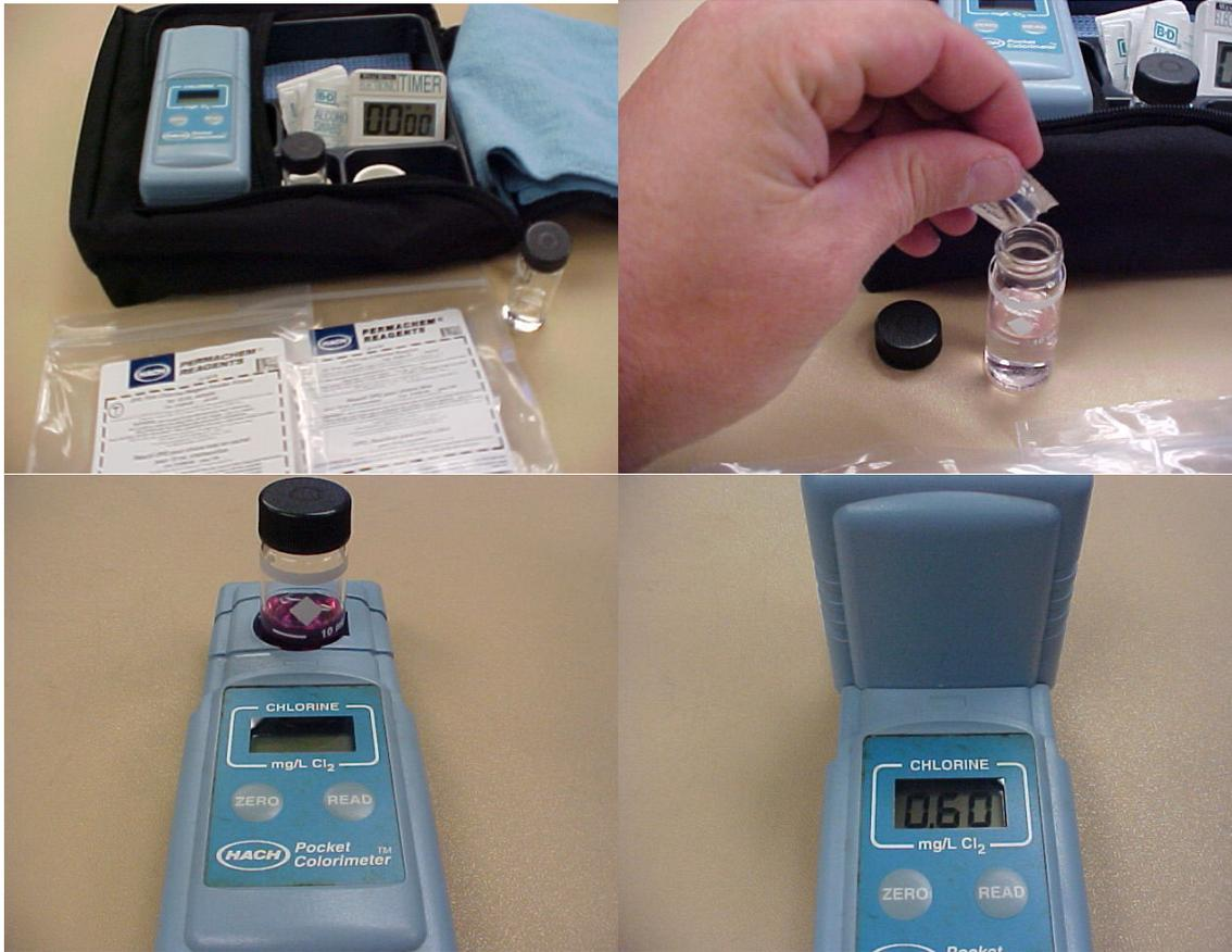
Small portable chlorine measuring kit. The redder the mixture the “hotter” or stronger the chlorine in solution.
