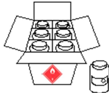
**Figure 4.13 Combination Packaging (Outer box with inner bottles)**
