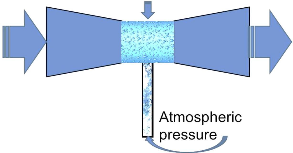
The newest injector design causes complete mixing of injected materials (air, ozone or chemicals), eliminating the need for other in-line mixers. Venturi injectors have no moving parts and are maintenance free. They operate effectively over a wide range of pressures (from 1 to 250 psi) and require only a minimum pressure difference to initiate the vacuum at the suction part. Venturis are often built in thermoplastics (PVC, PE, PVDF), stainless steel or other metals.
