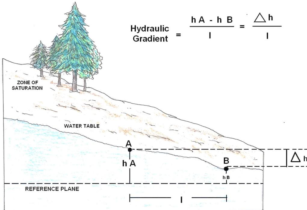
The *hydraulic gradient* is a vector gradient between two or more hydraulic head measurements over the length of the flow path. It is also called the 'Darcy slope', since it determines the quantity of a Darcy flux, or discharge. A dimensionless hydraulic gradient can be calculated between two piezometers as:
