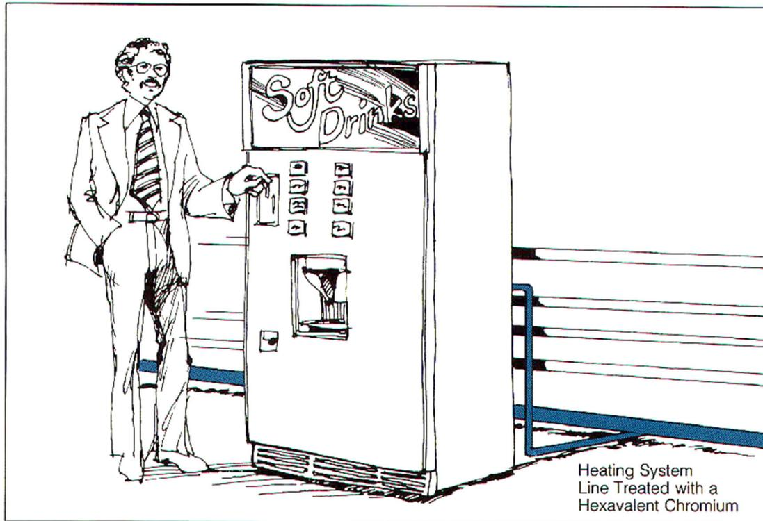
Several cross-connection have been made to soda machines, the one to worry about is when you have a copper water line hooked to CO<sub>2</sub> without a backflow preventer.
