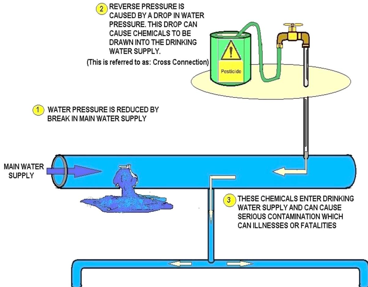
Above is one example of a commonly found cross-connection. This type of cross-connection happens every time the water pressure in the water main is reduced or shut-down.
