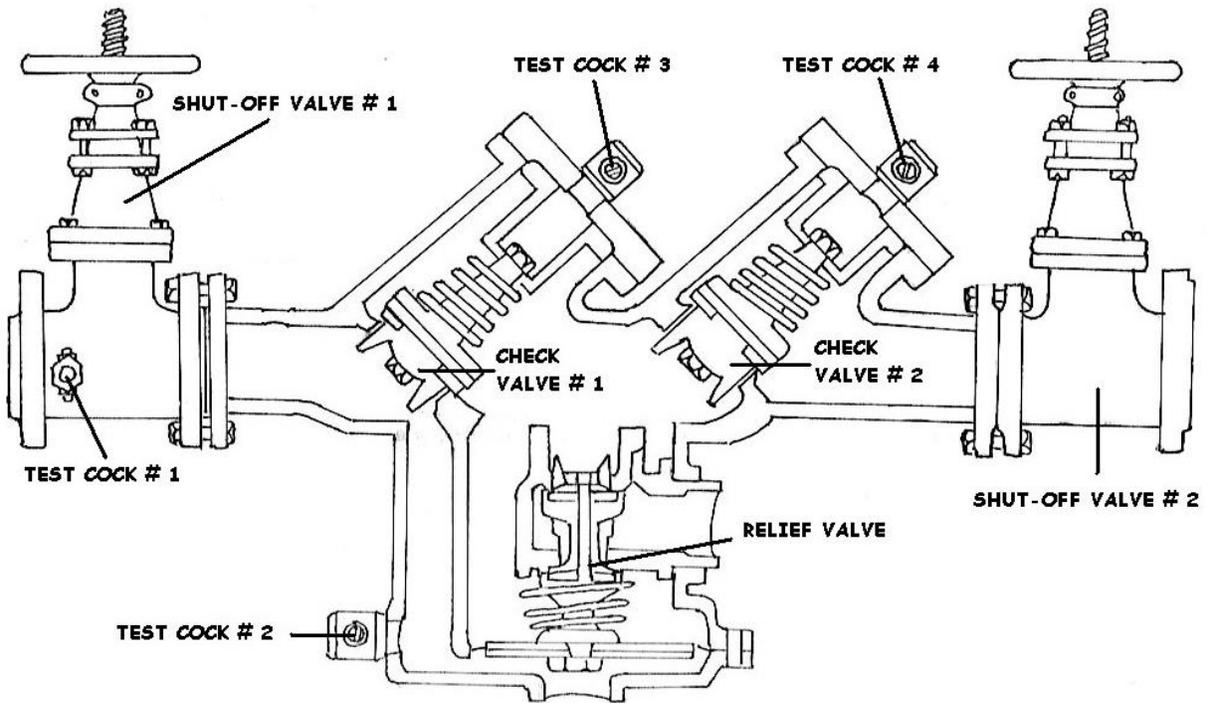
**REDUCED PRESSURE BACKFLOW PRINCIPLE ASSEMBLY**
