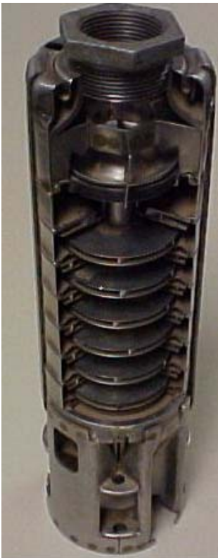
Cut away of a small submersible pump.
