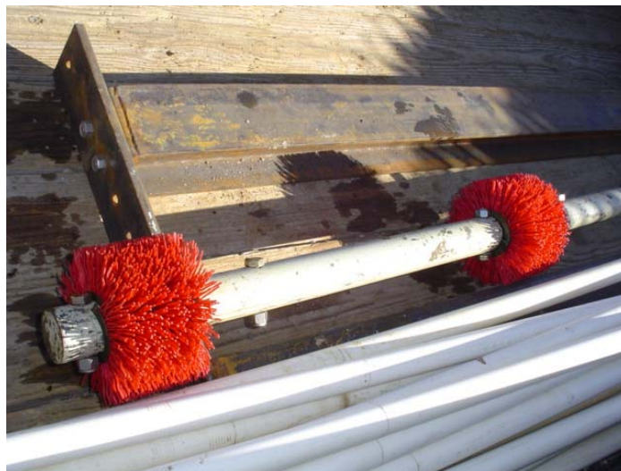
This brush is used to dislodge debris inside well casing.
