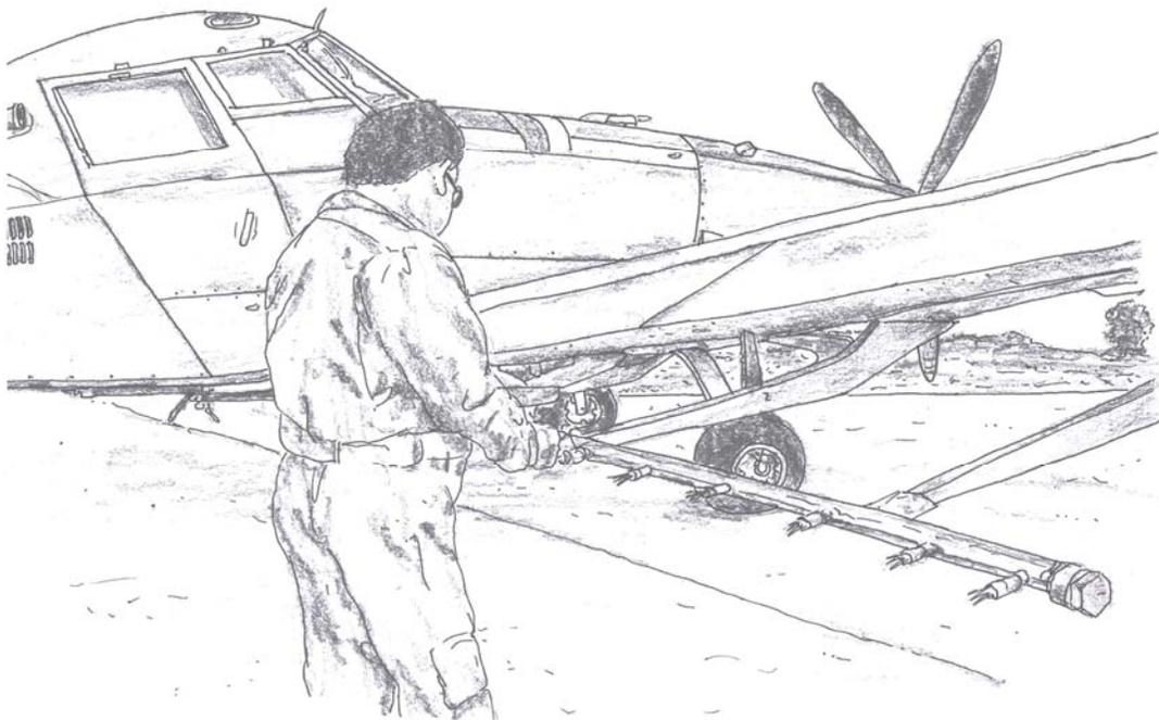
**PILOT DOING PRE-FLIGHT CHECKS ON NOZZLES**
